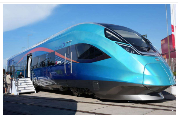
CRRC 2,000kW Hydrogen Fuel Cell Hybrid Locomotive
